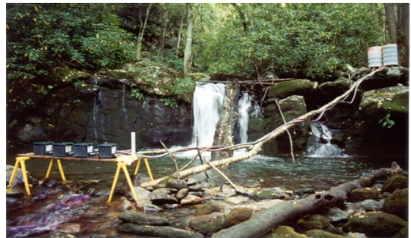
Figure 18. The potassium permanganate deactivation station used to neutralize antimycin during a native fish restoration project in GRSM.
