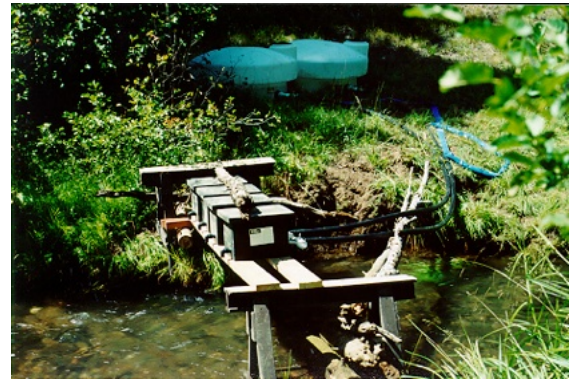
Figure 19. A Potassium permanganate deactivation station configuration used to detoxify antimycin during native fish restoration project in Crater Lake NP. Note large drums used for larger stream volume ( \sim 15 cfs).
