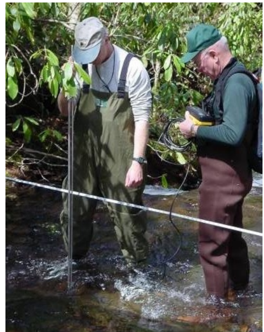
Figure 10. — Measurement of stream discharge using the cross sectional area method. Note personnel standing downstream of the meter.
