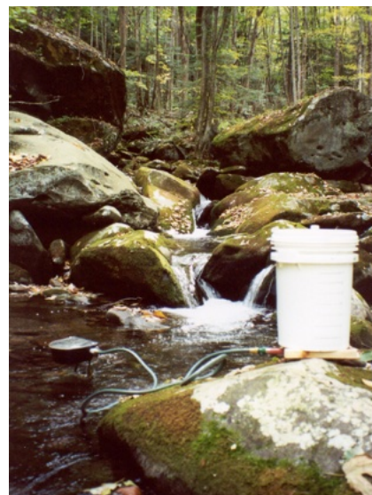
Figure 15. A Operational antimycin dispensing station on Sams Creek, GRSM during treatment in 2000.
