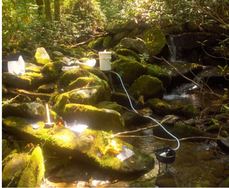
Figure 4. Antimycin A drip station in operation during a small stream treatment. The apparatus includes a dispensing bucket (19L or 5-gal) containing formulated product (water, antimycin A, and the surfactant nonoxyl-9). The dispensing bucket is calibrated to deliver 3.8L or 1-gal per hour.
