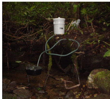
Figure 16. An operational antimycin drip station on Bear Creek, GRSM during the 2003 treatment.
