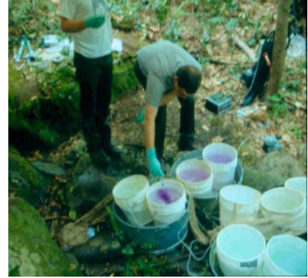
Figure 13. Setup of streamside bioassay tubs and buckets used to determine the target concentration of antimycin (ppb) and potassium permanganate (ppm)
