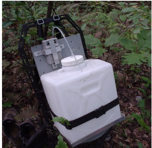
Figure 14. A backpack fish transporter and aerator used to transport sentinel fish to and from holding cages and the treatment area.
